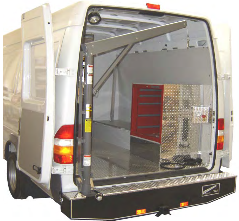
Shown with optional WO-16 Aluminum Diamond Plate Cover and WO-2 Left Side Mast Location (right side std.)
